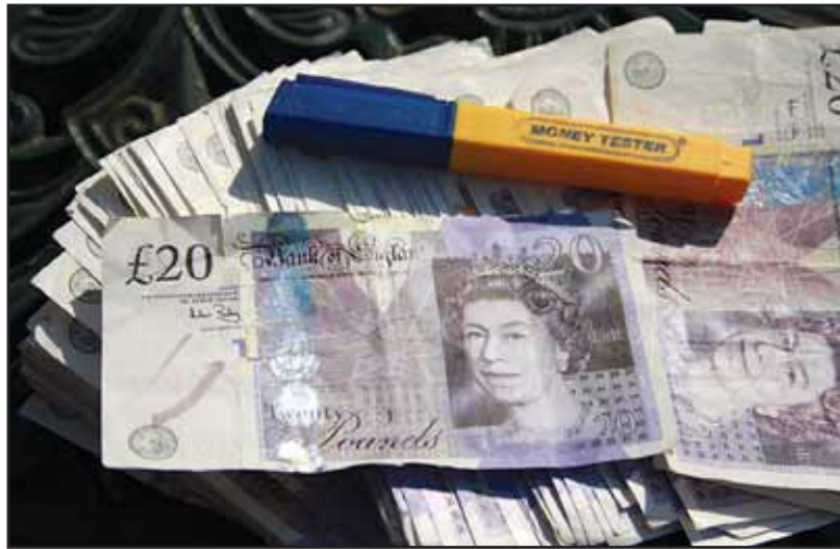
The mark made by the Money Tester pen on the left-hand side of the £20 note proves the note is a forgery.
